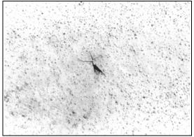
Coating damage can appear as gouges, cracks, and punctures. Hail induced coating cracks often form patterns shaped like "crow's feet" or semi-circles.
