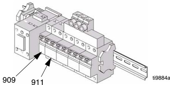
FIG. 10: Circuit Breaker Module
