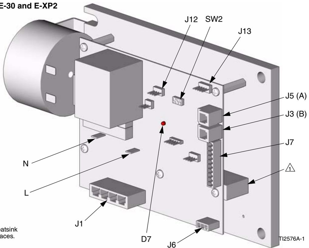
Apply 110009 thermal heatsink compound to mating surfaces.
